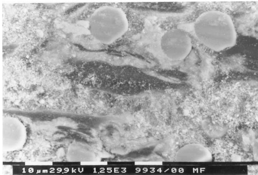
Figure 6 Worn surface hot-press cooled of GF/PA6 pin after 20,000 metres sliding in normal direction.
